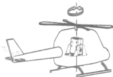
Helicopter (Yaw Stabilization) RX ⇒ PG-02 ⇒ Rudder Servo
